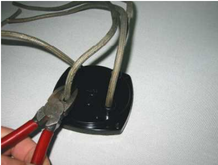
1. Remove existing harness wires.
