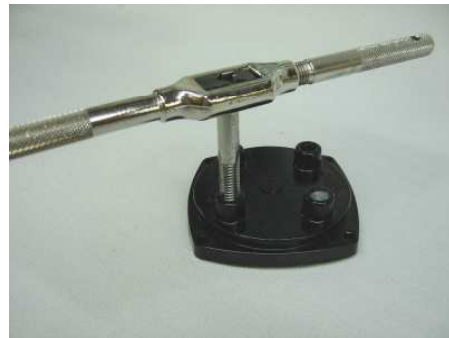
4. Tap hole to 3/8" x 16 coarse thread pitch. Chamfer holes each side. De-burr threads lightly.
