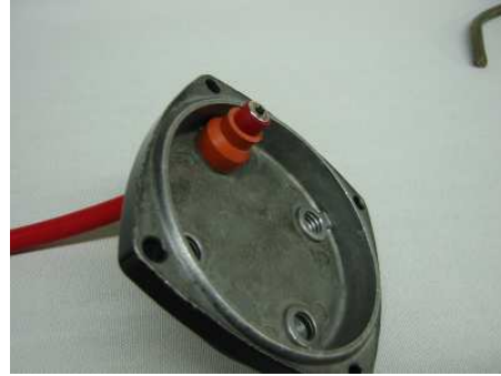
14. Install insulator nipple.
