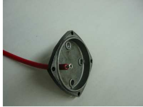
8. Install insert/rivet on center conductor.
