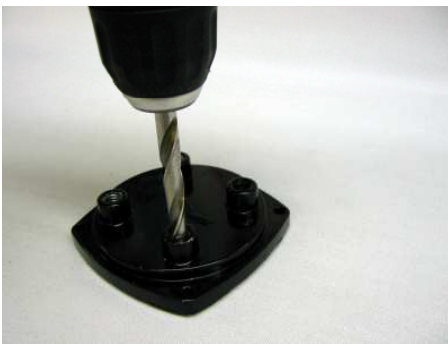
3. Drill holes to 5/16"
