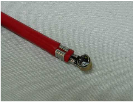
15. Properly crimped spark plug terminal end.
