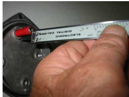
12. Adjust total height to .850" from the top of slight rise in cap.
