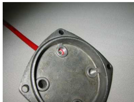
6. Use silicone RTV on the cap thread to act as lubricant/adhesive. Very slowly screw wire into cap. Do not twist/tear the wire. If you break the fiberglass core, it will be heard and felt. This small section of damaged wire must be cut-off and removed, start over.
