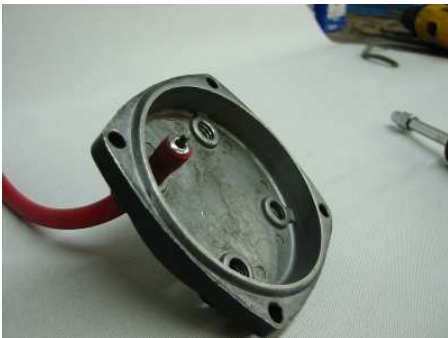
11. Seat completely and cut off center conductor flush.
