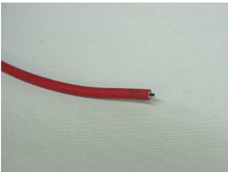
5. Trim wire to leave a 1/8" of center conductor protruding.
